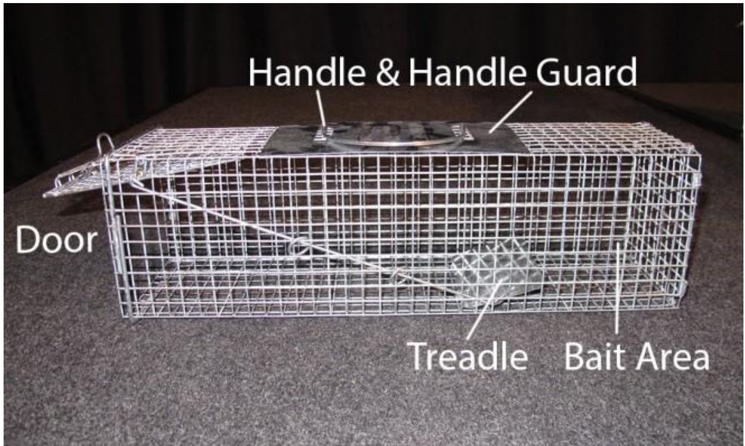
The anatomy of a box trap. (Photo by Stephen M. Vantassel)
